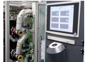
Synthetic-gas test bench for performance characterization of exhaust catalysts.
