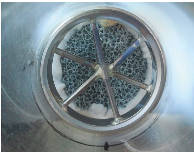
Tube reactor with open-celled ceramic foam as catalyst (source: Fraunhofer ICT).
